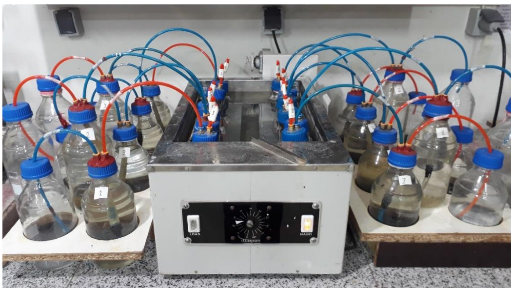
Fig. 2. Biochemical methane potential (BMP) testing system.
