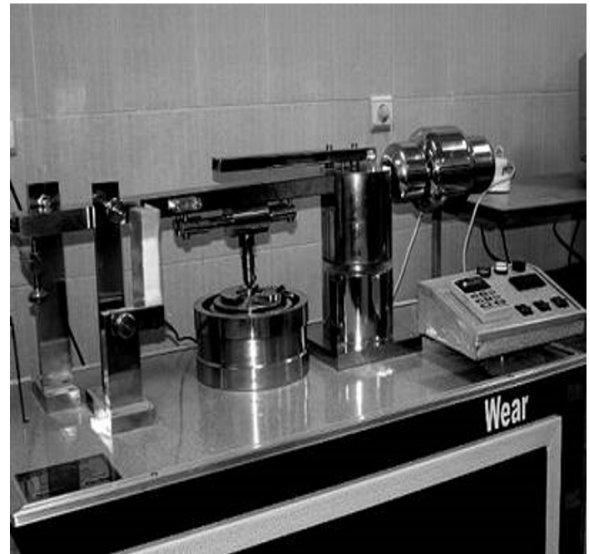
Fig. 1. A view of the pin-on-disc tribometer and the schematic of its operation.
