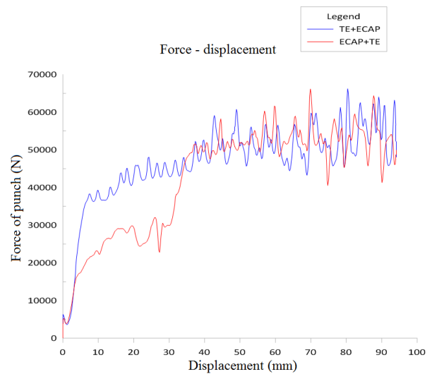
Fig. 5. Corresponding force-displacement diagram for two extruded samples.
