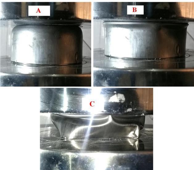
**Fig. 8.** Crushing process of sample S2 (thickness of 2mm): a) Start of crushing test, b) Start of buckling in the sample, and c) Sample after crushing.
