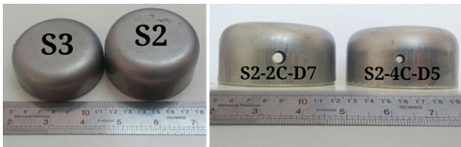
**Fig. 5.** Sandwich deep drawn cups without edges; a) Without trigger, and b) With circular cutout triggers.
