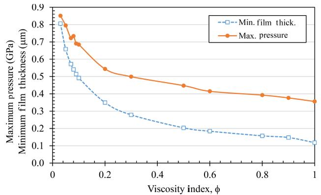
**Fig. 7.** Grease film thickness and maximum pressure to plastic viscosity,  $\phi$ .
