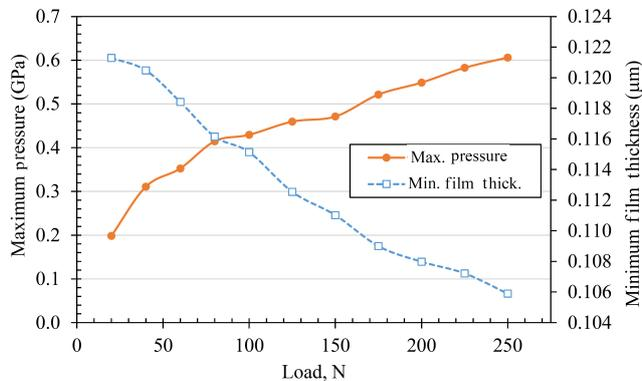
**Fig. 8.** Load effect on film thickness and maximum pressure.
