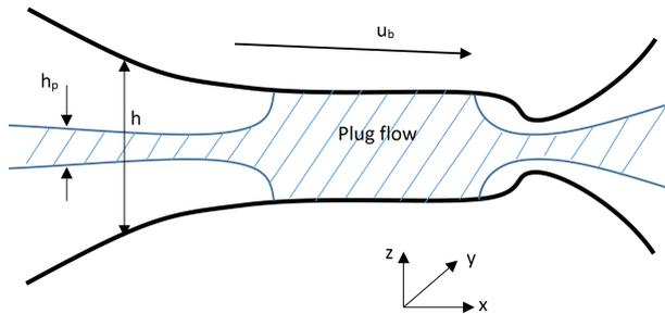
**Fig. 1.** Contact geometry in elastohydrodynamic lubrication and non-Newtonian grease lubricants.
