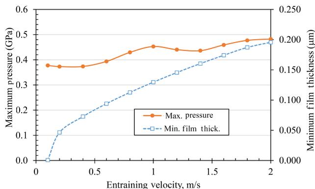
**Fig. 9.** Speed effect on film thickness and maximum pressure.
