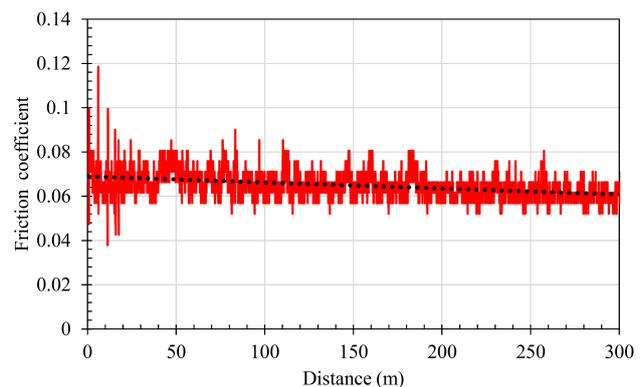
Fig. 3. Experimental results of friction coefficient in 20N load and 0.23m/s velocity condition.
