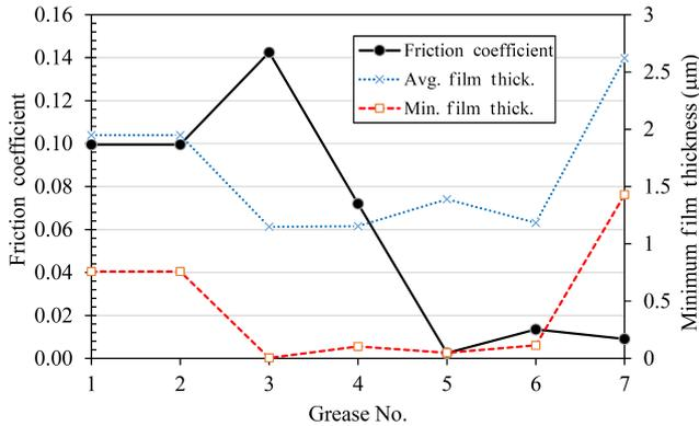
**Fig. 5.** Friction coefficient and film thickness for various type of lubricants, at 100N load and 1m/s entraining velocity.
