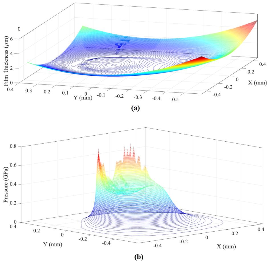
**Fig. 4.** The pressure distribution and film thickness in contact area for 200N load and 0.8m/s velocity.
