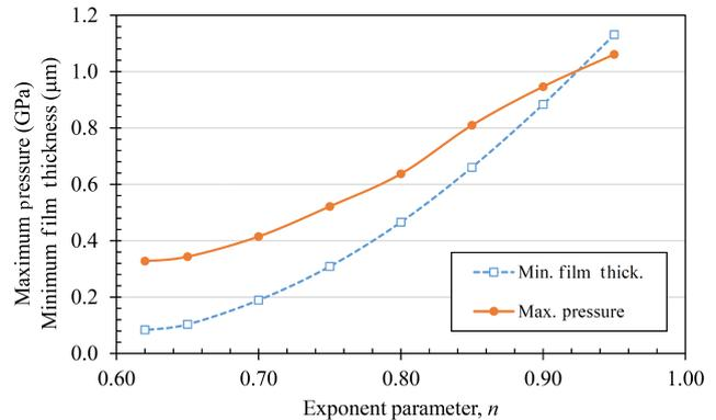
**Fig. 6.** Grease film thickness and maximum pressure to rheological exponent,  $n$ .
