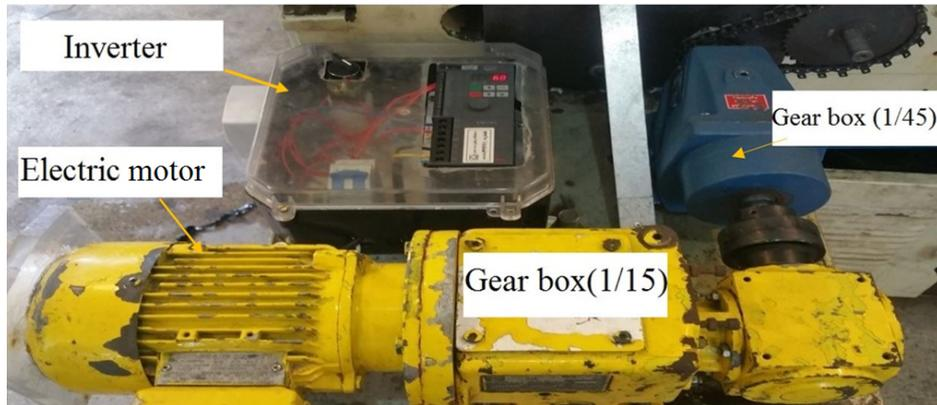
**Fig. 1.** Moving system of longitudinal feed for the grinding machine.**Table 3**
