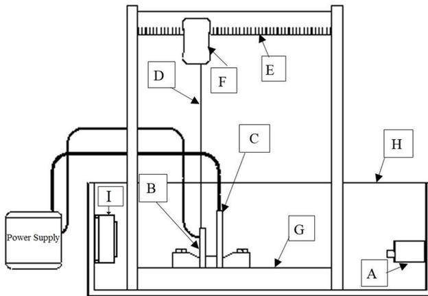
**Fig. 3.** The scheme of the electropolishing layer removal measurement system; a) Pump, b) Specimen (anode), c) Cathode, d) pointer, e) Scale, f) Camera (in front of the pointer), g) Holder, h) Tank, and i) Cooling system.
