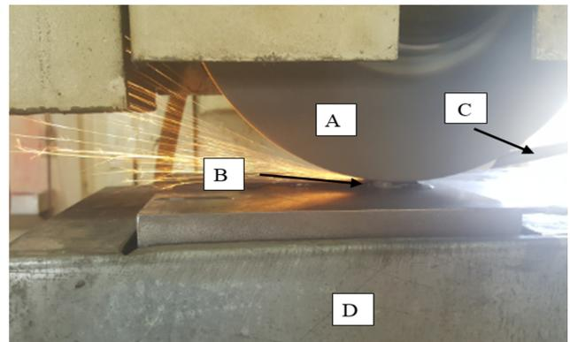
**Fig. 2.** Creep-feed grinding set-up, a) Grinding wheel, b) Specimen, c) Coolant nozzle, d) Dynamometer.
