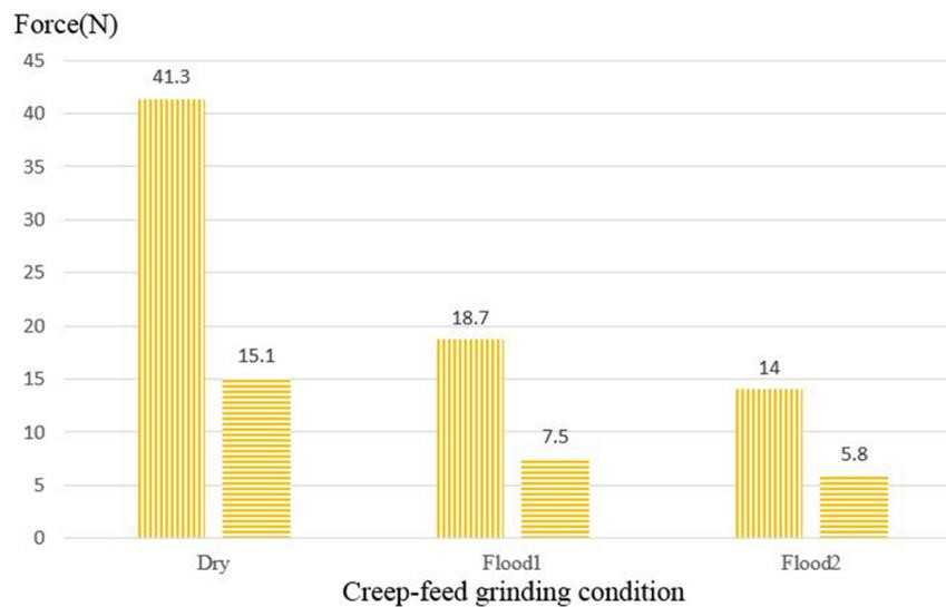
**Fig. 4.** Measured average tangential and normal creep-feed grinding forces at different cooling conditions.
