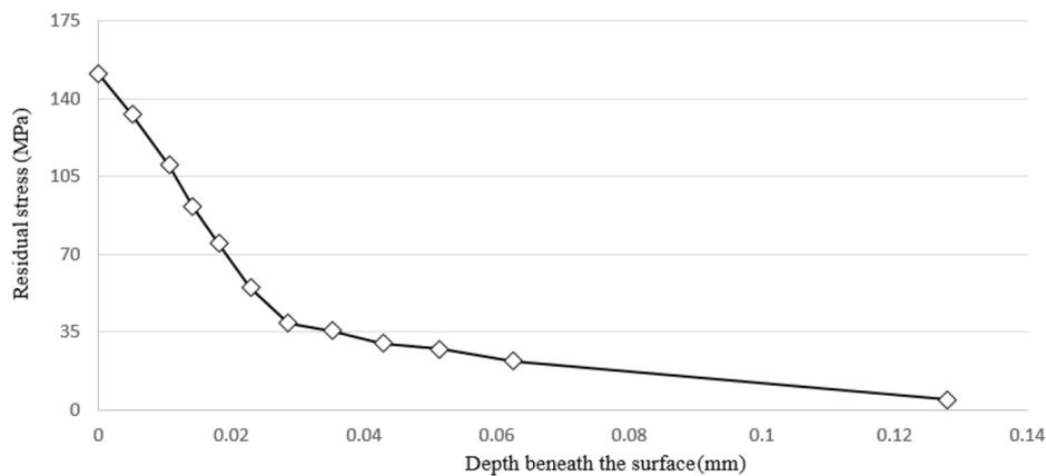
**Fig. 7.** The values of residual stresses along the depth of the specimen during creep-feed grinding for the flood 2 condition.
