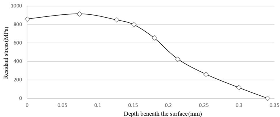
**Fig. 5.** The values of residual stresses along the depth of the specimen during creep-feed grinding for the dry condition.
