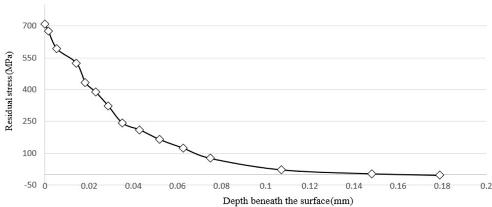
**Fig. 6.** The values of residual stresses along the depth of the specimen during creep-feed grinding for the flood 1 condition.
