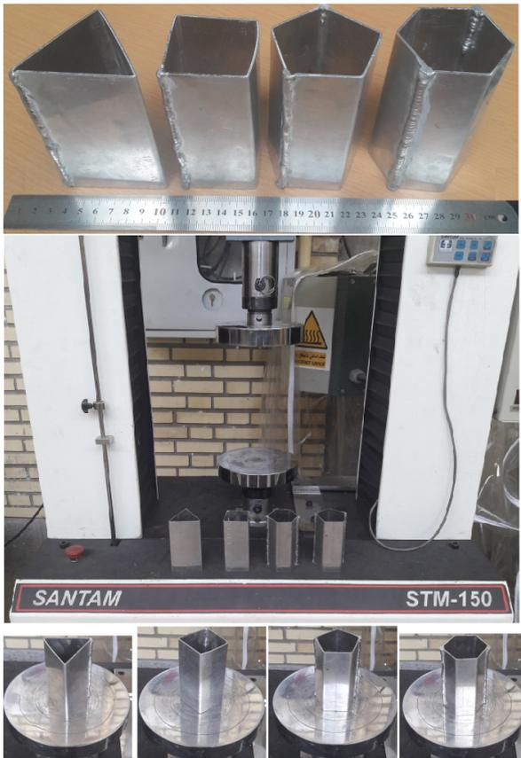
**Fig. 3.** Prepared test specimens for verifying the simulation results.
