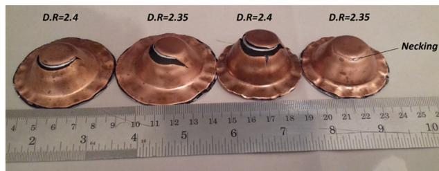
**Fig. 9.** Experimental samples with rupturing and necking.
