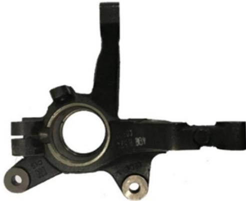
**Fig. 6.** Front steering knuckle in driver’s side of a four cylindrical passenger car.
