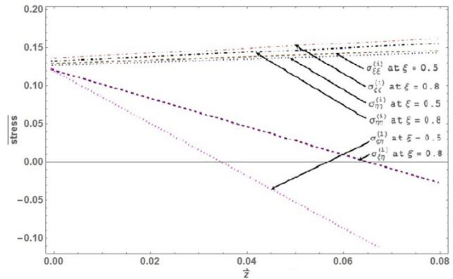
Fig. 4c. Stresses along the axial direction.
