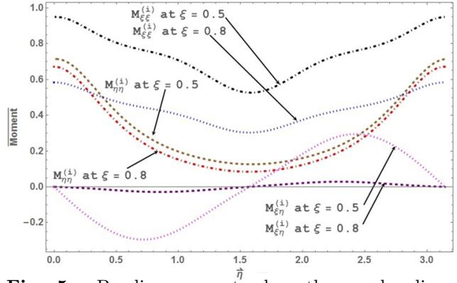
Fig. 5a. Bending moments along the angular direction.
