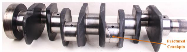
**Fig. 2.** Photograph of the broken down crankshaft at the second crankpin.
