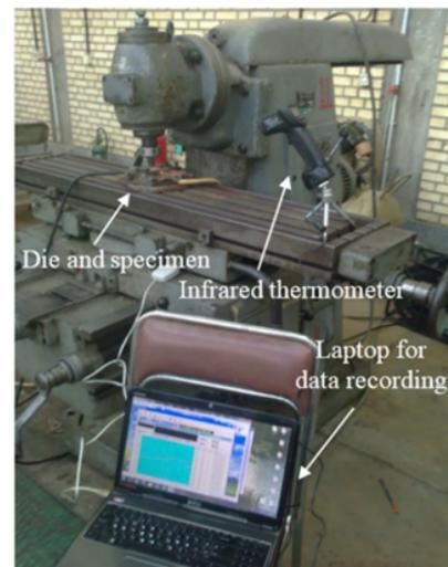
**Fig. 4.** Thermometer installed on the table of angle grinder for measuring instantaneous temperature.
